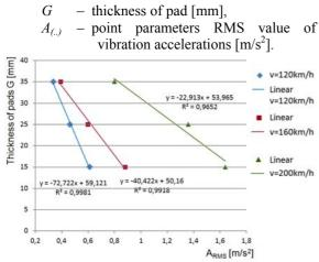
Fig. 10. Dependence of pad's thickness in function of point parameters ( $A_{RMS}$  value) of vibrations accelerations for measurement in the  $Y_I$  direction for speed at the beginning of braking v=120, 160 and 200km/h
