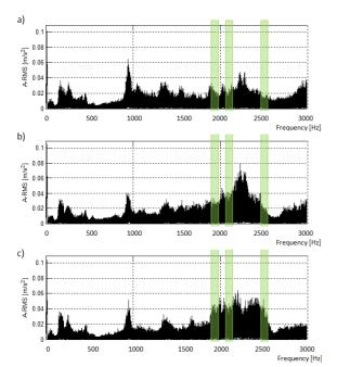
Fig. 6. Dependence of amplitude of vibration accelerations on frequencies for different pad's thicknesses during braking from speed of 160km/h in direction Y1: a) pad's thickness G1=35mm, b) pad's thickness G2=25mm, c) pad's thickness G3=15mm
