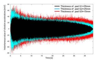
Fig. 4. Signal of vibration accelerations registered on pad caliper in direction  $Y_1$  for different thickness of pads during braking to stop (Speed at beginning of braking v=120km/h)
