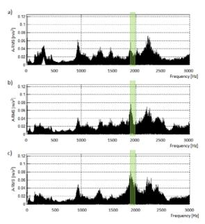
Fig. 7. Dependence of amplitude of vibration accelerations on frequencies for different pad's thicknesses during braking from speed of 200km/h in direction Y1: a) pad's thickness G1=35mm, b) pad's thickness G2=25mm, c) pad's thickness G3=15mm
