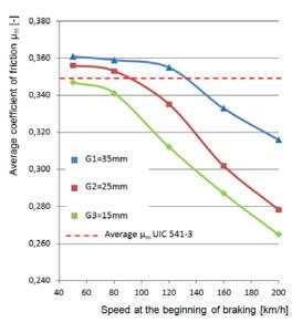
Fig. 8. Dependence average coefficient of friction of speed at the beginning of braking for three thickness of friction pads
