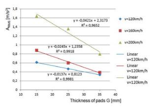
Fig. 9. Dependence of pad's thickness in function of point parameters ( $A_{RMS}$  value) of vibrations accelerations for measurement in the  $Y_1$  direction for speed at the beginning of braking v=120, 160 and 200km/h
