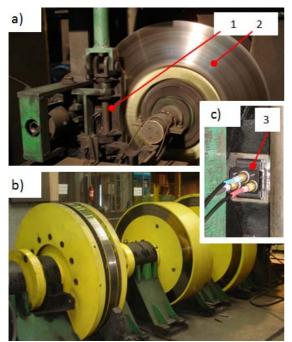
Fig. 2. Interial station for tests of railway brakes: a) view of level set of railway disc brake, b) view of masses using to brake simulated load to passenger car, c) accelerometer B&K 4504A; 1- calliper with brake pads, 2- disc brake type 590×110, 3- accelerometer
